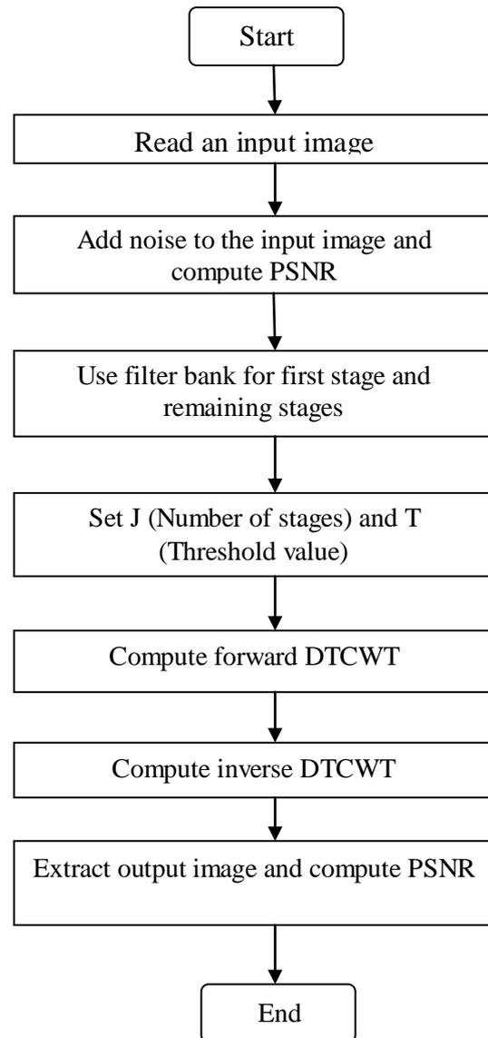
Fig. 4 Flowchart of Dual-Tree Complex DWT
