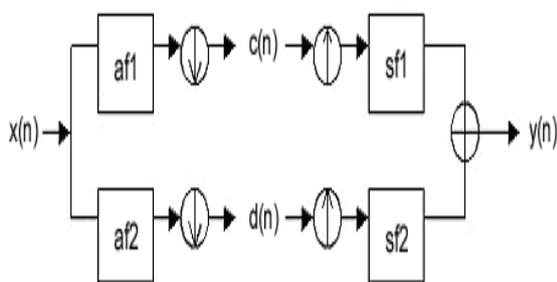
Fig. 1 One dimensional filter bank
