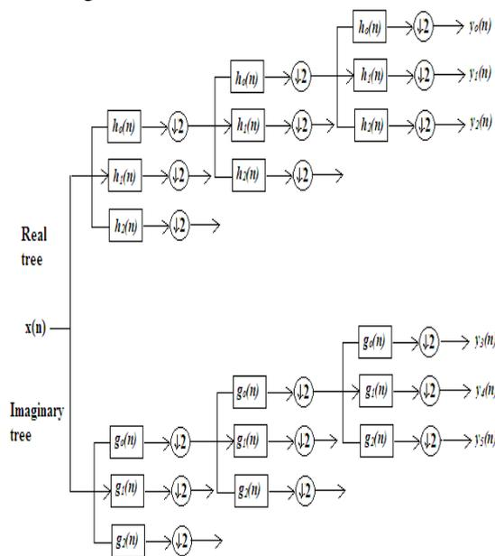
Fig. 5 Design implementation of the Double-Density Dual-Tree Complex DWT
