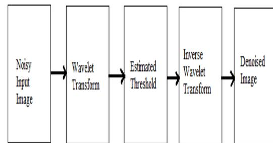
Fig. 2 A block schematic of wavelet based image denoising technique
