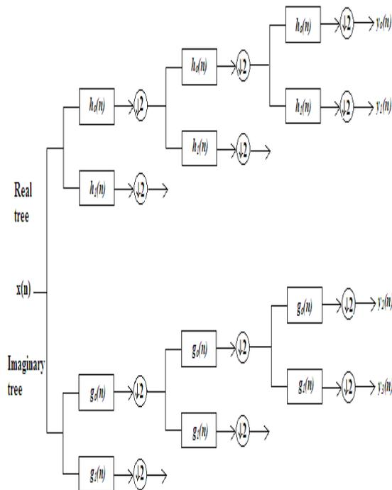
Fig. 3 Design implementation of Dual-Tree Complex DWT
