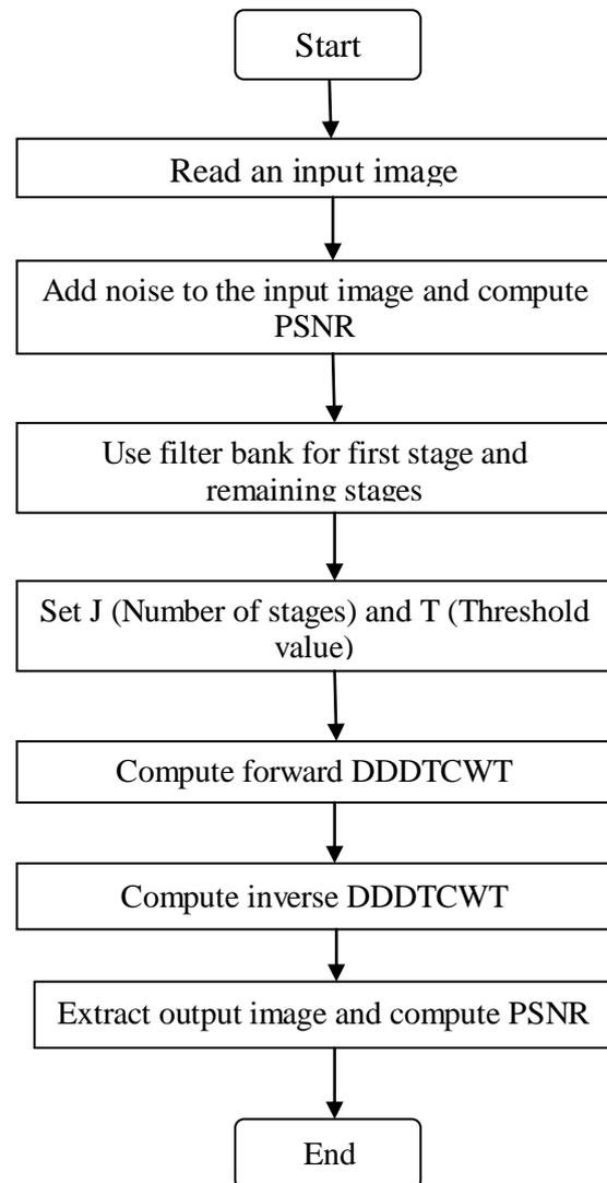
Fig. 6 Flowchart of Double-Density Dual-Tree Complex DWT
