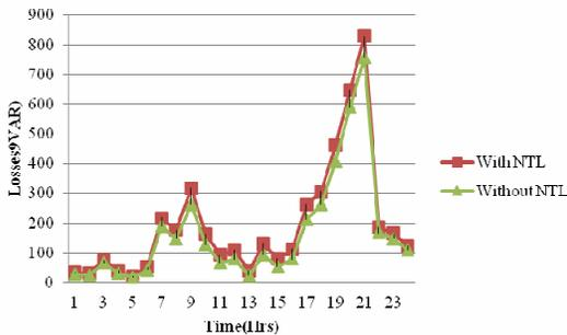
Fig.4.2 Comparison of reactive power losses
