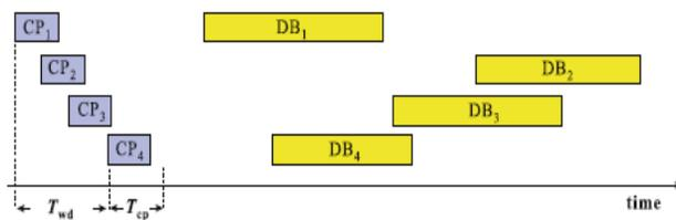
Figure 3.3 Transmission of data bursts in OBS
