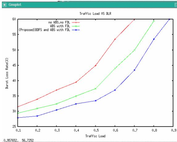
Figure 4.8 Traffic Load vs. BurstLossRate
