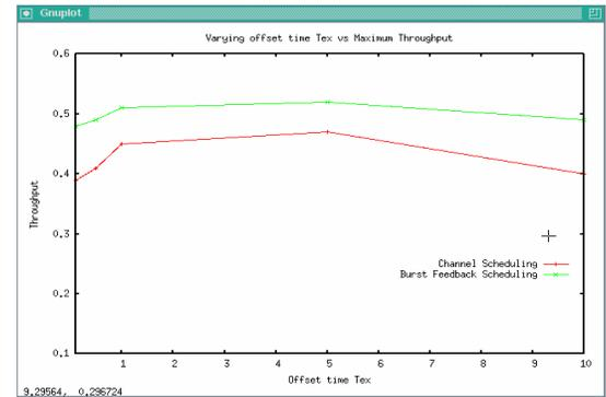
Figure 4.6 Offset Time vs. Throughput
