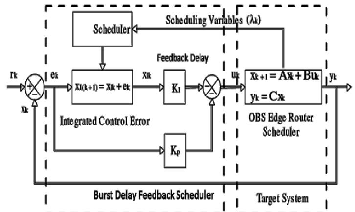
Figure 3.4. A linear control system with feedback control mechanism using burst delay feedback scheduler.
