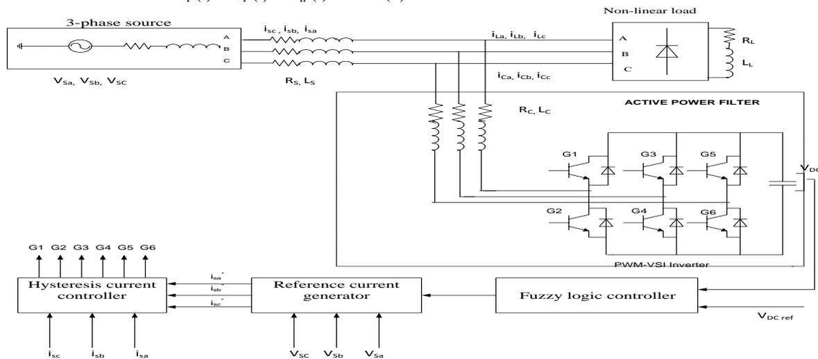
Fig1. Block diagram of Shunt Active Power Filter with proposed FLC
