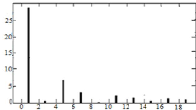
Fig10. FLC based APF; Order of harmonics, The source current without active filter (THD=28.61%),
