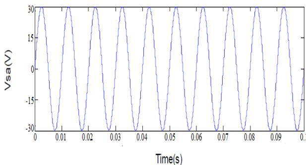
Fig6. Source voltage before compensation
