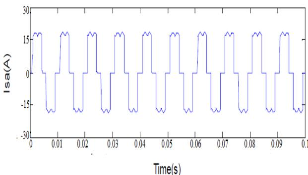
Fig7. Source current before compensation
