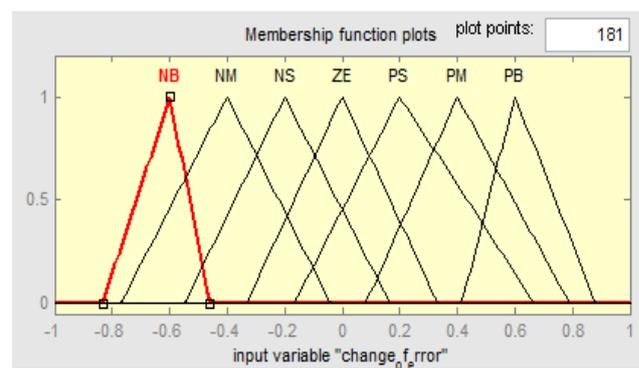
Fig4. Triangular membership function for input variable 'change of error'
