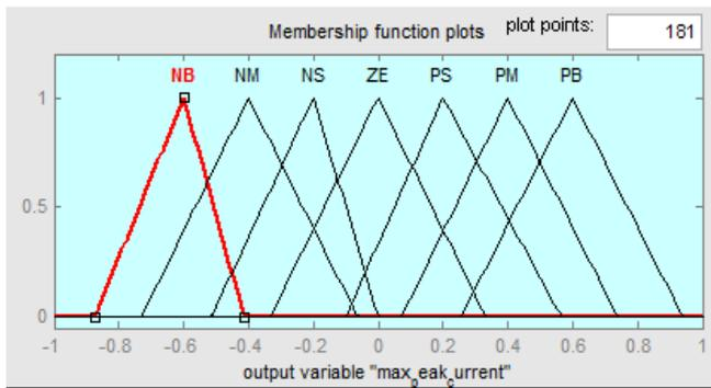
Fig5. Triangular membership function for output variable 'maximum current'
