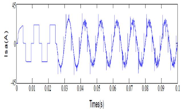
Fig8. Source current after compensation
