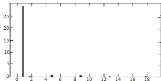
Fig11. FLC based APF; Order of harmonics, The source current with active power filter (THD=3.85%)
