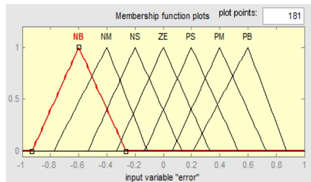
Fig3. Triangular membership function for input variable 'error'
