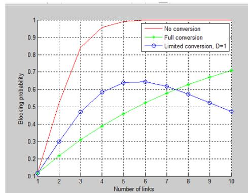
Fig.2: Blocking Probability for 10 links when load is 10 Erlangs per link
