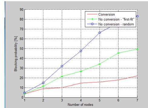
Fig 1: Blocking Probability for 10 links when load is 10 Erlangs per link .
