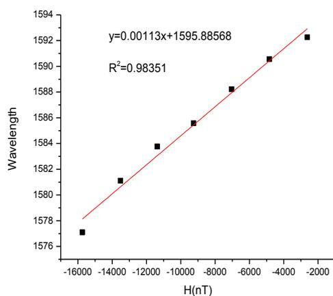
Figure 4: Relationship between wavelet and magnetic field strength
