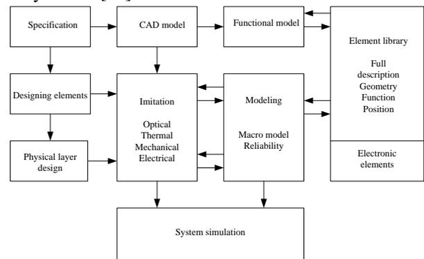
Fig. 1 Structural diagram of complex microsystem devices design
