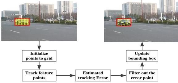
Fig. 1 Implementation process of the median flow tracking algorithm
