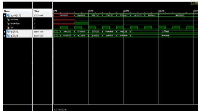
Fig.7: Floating point adder without pipelining unit
