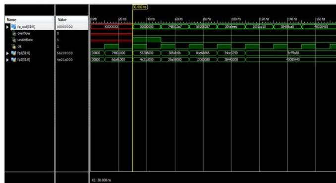
Fig.8: Floating point adder with 2 stage pipelining unit
