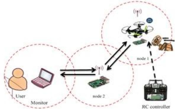
c- Node-2 Bridge Between Node-1 and Monitor
