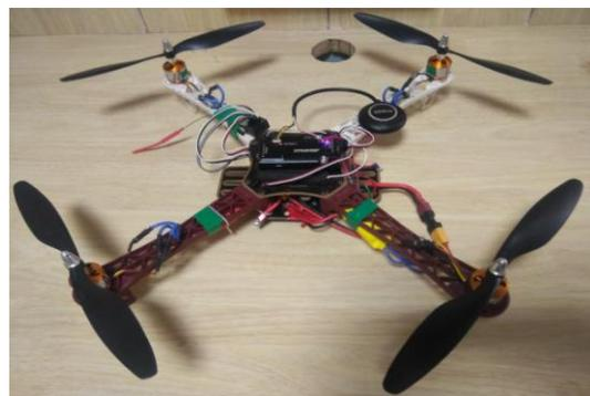
Fig.7 Quadcopter using APM 2.8 board
