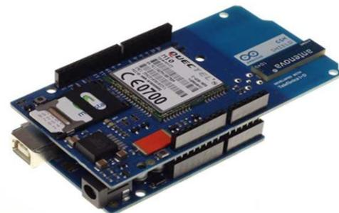
Fig. 4, “Arduino GSM Shield” [13]
