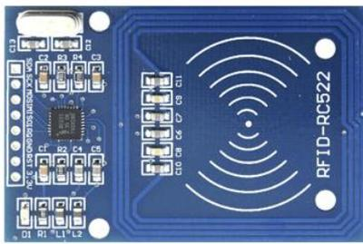
Fig. 5, “RC522 RFID module” [14]
