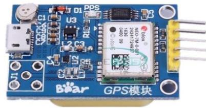
Fig. 3, “Arduino GPS Shield” [12]
