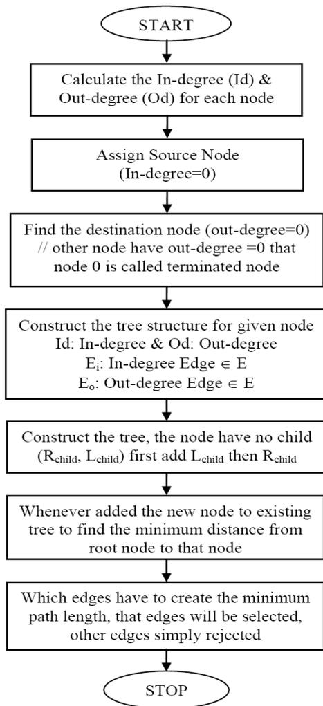
Figure 4. Flow diagram for BTSNA-DS.
