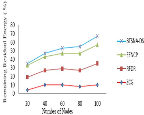
Figure 10. Remaining Residual Energy Vs. Number of Nodes.
