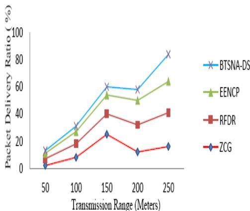
Figure 14. Packet Delivery Ratio Vs. Transmission Range (Meters).
