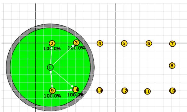
Figure 3: Network Topology of Smart Trash Pool System. Node 1 which is green is sink and other nodes in yellow are trash nodes. The green area is the Transmission Range (Tx) and area in grey is the Interference Range (INT) of the sink node. The distance between nodes d= 30m
