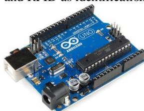
**Fig.2. Arduino Uno Board [11]**
