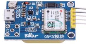
**Fig.3. Arduino GPS Shield [12]**
