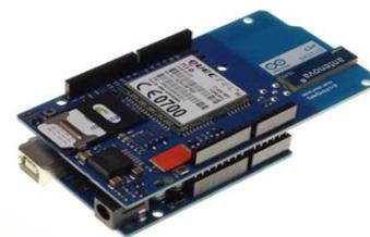
**Fig.4. Arduino GSM Shield [13]**
