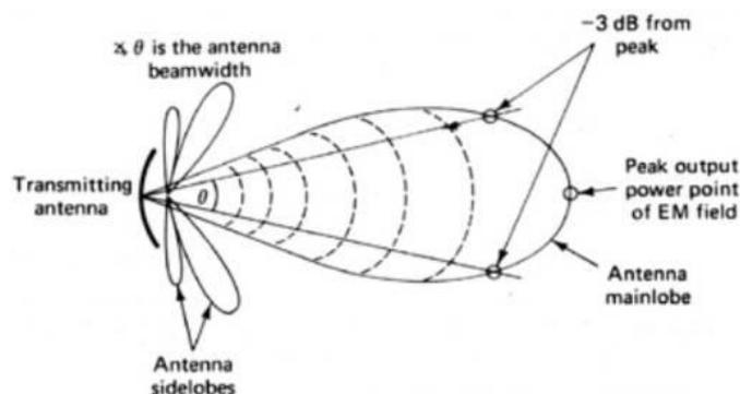
Fig.1 Structure of Electromagnetic beam
