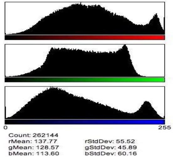
Figure (1): Color histogram diagram of three channels (Red, Green and Blue).
