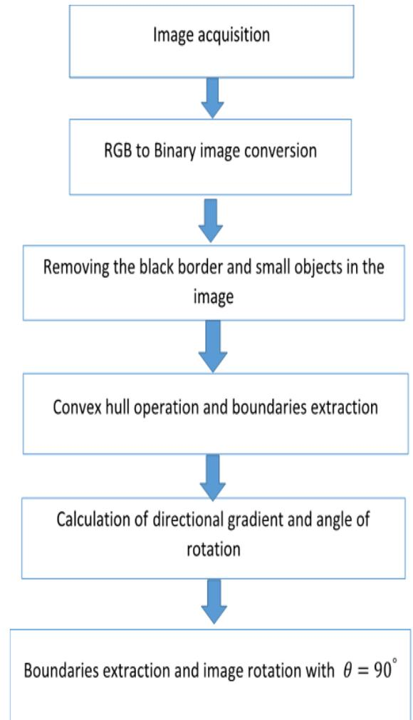
Figure (4): Image object extraction block diagram.
