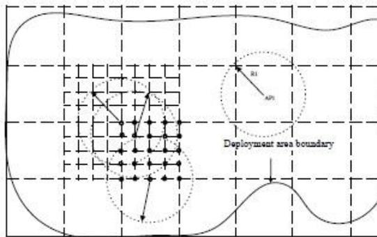
Fig 2. Efficient AP deployment in grid cell
