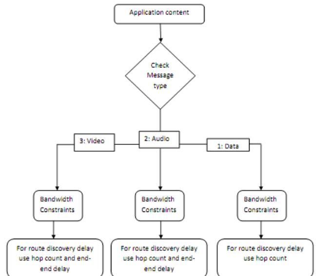
**Figure 2: Flowchart for Proposed System Model**
