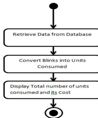
The Cost Display Module displays the Number of Units used by consumer and its cost. This module gets the blink count from the Server and converts them to Unit from which the cost is calculated. For example if the meter has a 1000 imp/Kwh then for every 1000 LED blink the user would have consumed 1 unit of electricity , which will be displayed in the main screen along with the cost.
