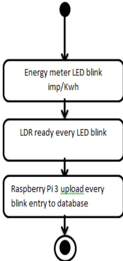
This part of the system does not need any user action it is automated. The LED blinks from the Energy meter is recorded by the Light Dependent Resistor which is connected to the Raspberry Pi 3. Every blink is uploaded to the SQL database by the Raspberry Pi 3 with a python code.
