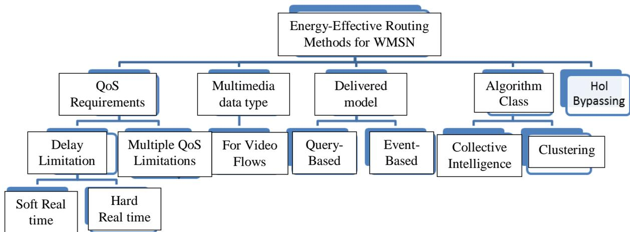
Fig1. Categorization of energy-effective routing algorithms for WMSN.
