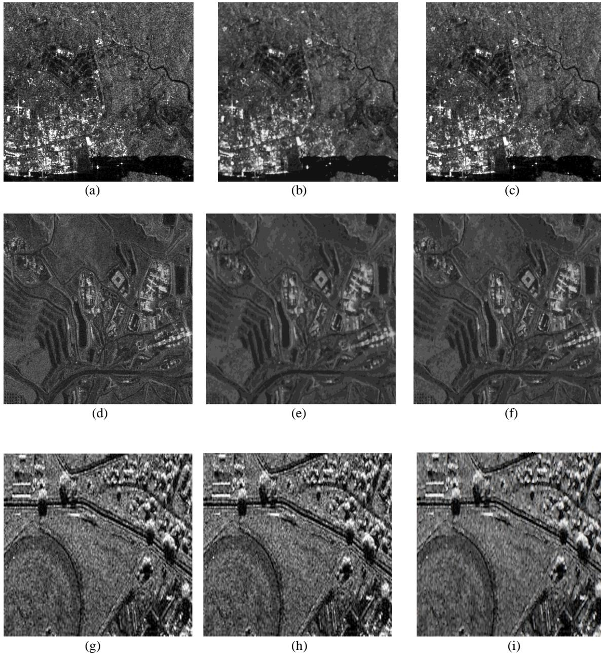
Fig.1. a) Noisy urban area image, b) De-speckling urban area image with NLM, c) De-speckling urban area image with adaptive NLM, d) Noisy terrestrial area image, e) De-speckling terrestrial area image with NLM, f) De-speckling terrestrial area image with adaptive NLM, g) Noisy vegetation area image, b) De-speckling vegetation area image with NLM, c) De-speckling vegetation area image with adaptive NLM
