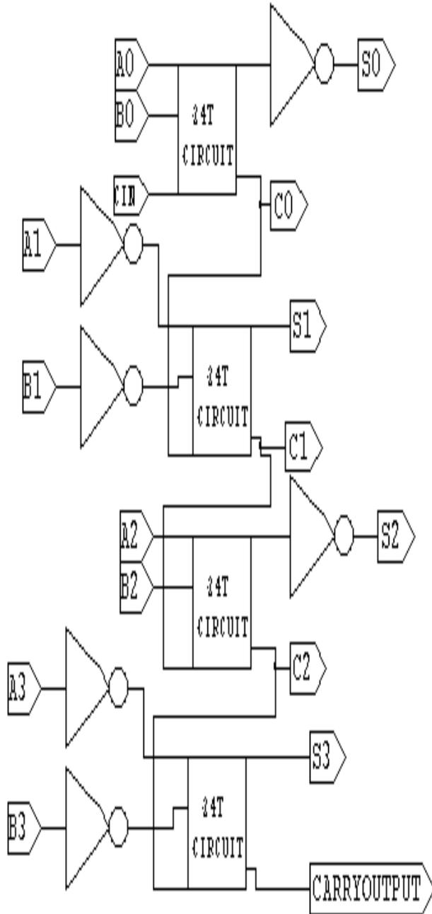
Fig. 3 Proposed 4-Bit Ripple Carry Adder Extendable to N-Bit.
