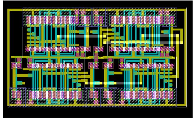
Fig. 4 Full custom layout of the 4-bit Ripple Carry Adder
