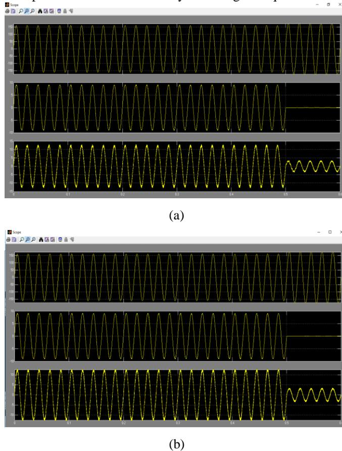
Fig. 3. Simulation waveforms of load voltage  $V_{ca}$ , grid current  $i_{ga}$ , and inductor current  $i_{La}$  when DG is transferred from the grid-tied mode to the islanded mode with: (a) conventional hybrid voltage and current mode control, and (b) proposed unified control strategy.
