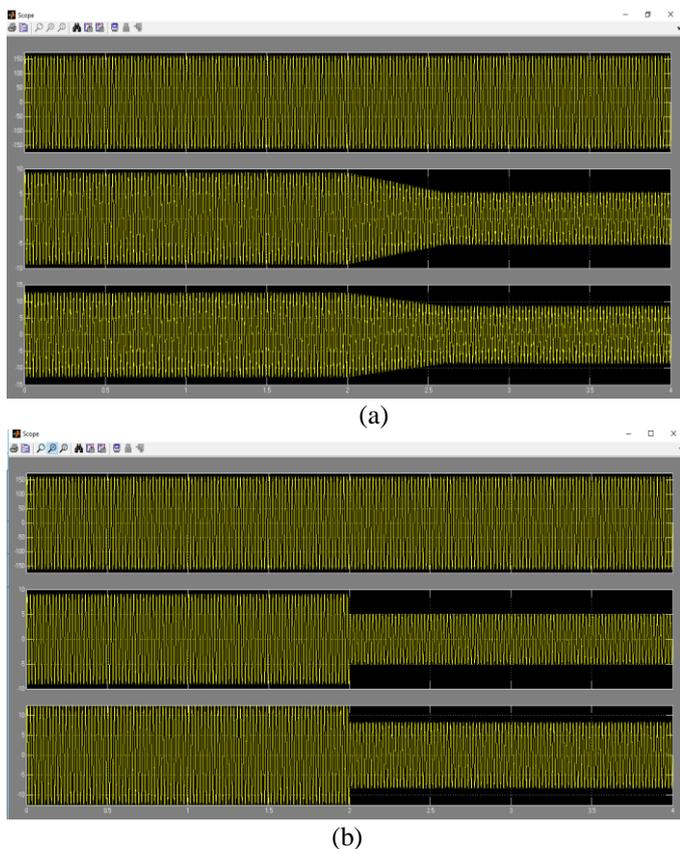
Fig. 2. Simulation waveforms of load voltage  $V_{ca}$ , grid current  $i_{ga}$ , and inductor current  $i_{La}$  when DG is in the grid-tied mode under condition of the step down of the grid current reference from 9 A to 5 A with: (a) conventional voltage mode control, and (b) proposed unified control strategy.
