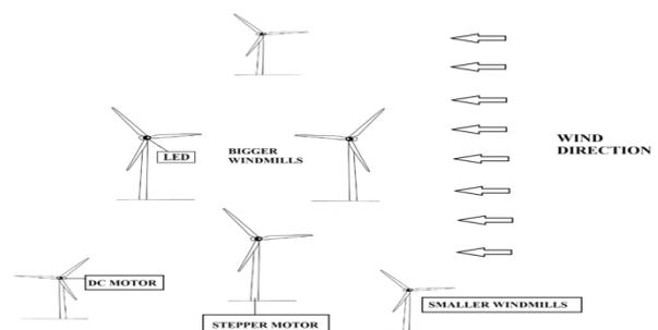
In this method small windmills are used to identify the direction of the wind. DC motors are installed at the apex of the turbine blades. Whenever dc motor rotates back EMF gets generated (Len’s law) which induces the current. The amount of current indicates the direction of wind. This information is passed to Arduino. MC will send signal to the stepper motors which are installed at base of the blades. The stepper motor rotates the bigger windmills towards the direction of wind flow
