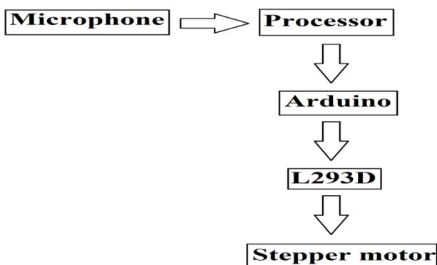
Fig.6. Block Diagram of Anemometer using Electret Microphone
