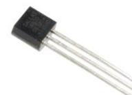
Fig 4.2 Temperature sensor
