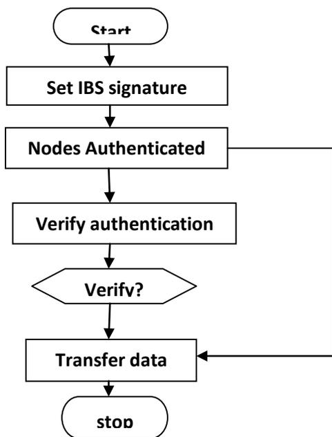
Figure 7: Flow chart of malicious node detection and data transmission
