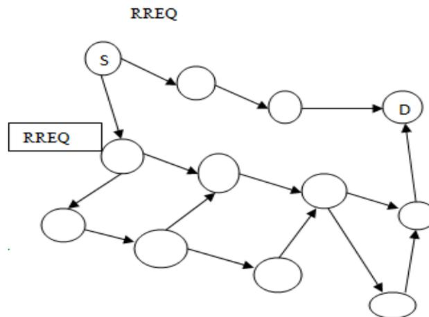
Figure 5: Transmission and Retransmission of RREQ message from source node S to neighbor nodes to find the route to the destination D.
