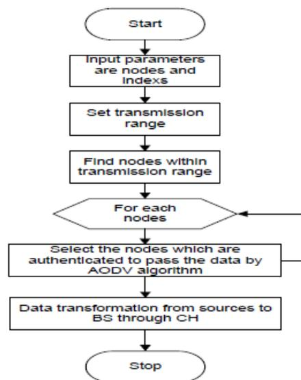
Figure 8: Flow chart of Secured Data Transmission in Network.
