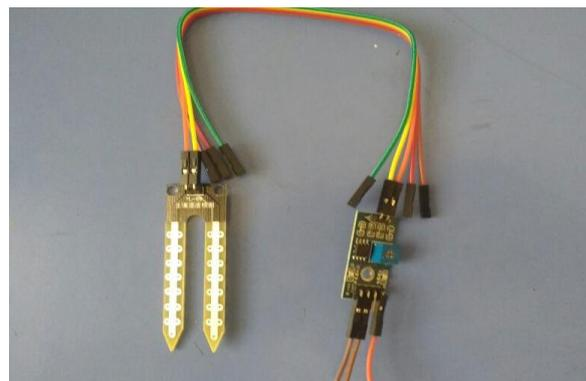
Figure 3: Y1-69- Soil Moisture Sensor
