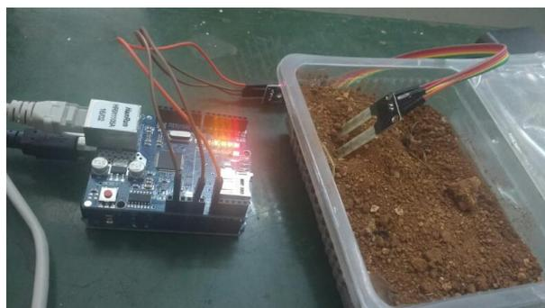
Fig 5 : YL-69 sensor in soil attached to Arduino
