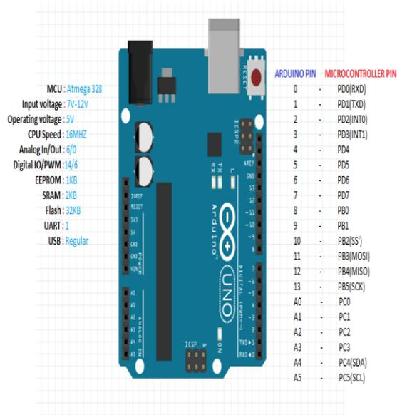
Figure 4: Arduino Uno Board
