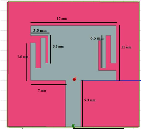
Fig 1. F slotted UWB microstrip Antenna
