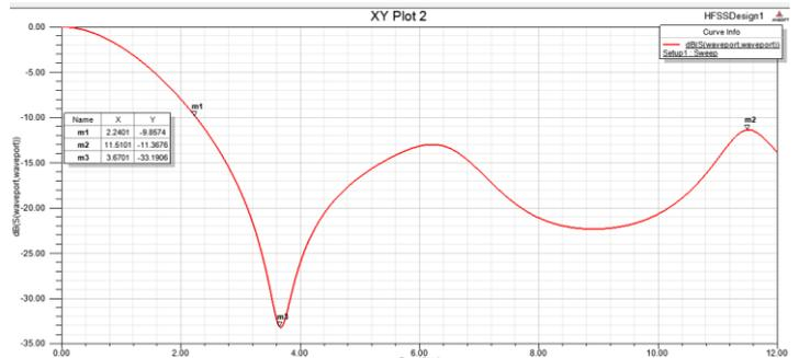
Fig 3 Return Loss Vs Frequency Plot
