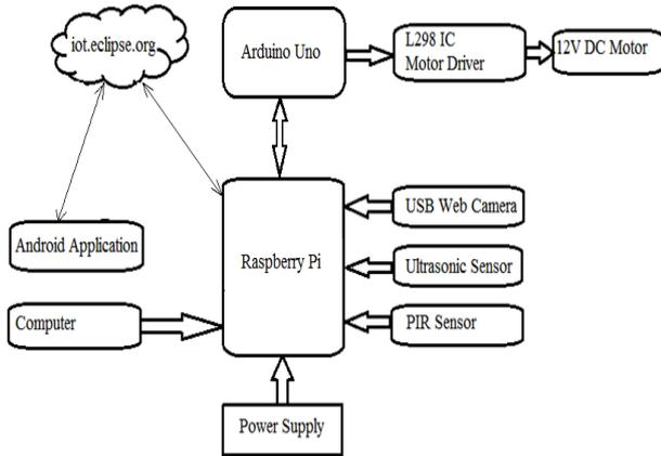
Fig.1 System Design for Smart Intruder Detection
