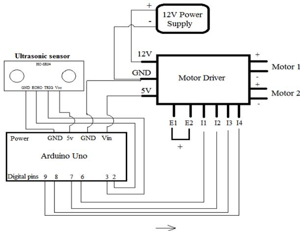
Fig. 4 Circuit diagram for Robot construction
