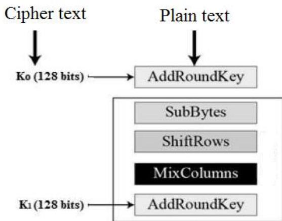
Fig 5: Operation involved in AES algorithm
