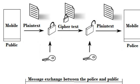
Fig 4: Message encryption using AES
