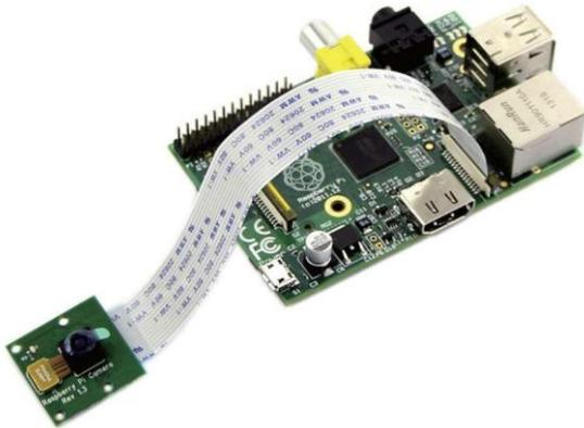
Fig II: Raspberry Pi with camera module connected
