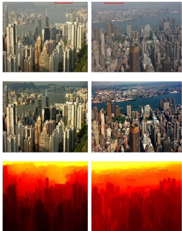
Figure 2: Haze removal results. Top: input haze images. Middle: restored haze-free images. Bottom: depth maps.
