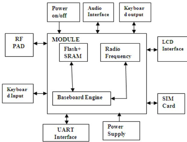
Fig.II: GSM module structure
