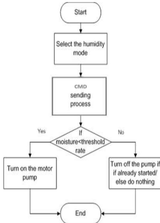
Fig.IV.Flow Chart of Humidity Mode
