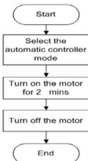
Fig.V.Flow chart of Automatic Mode
