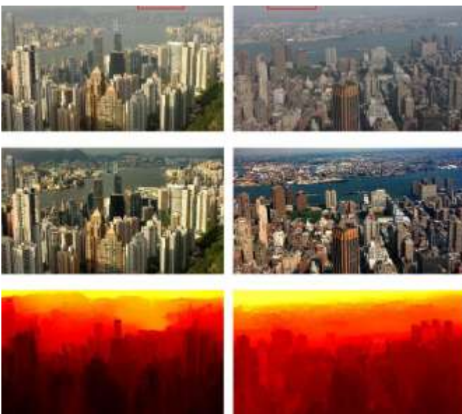
Figure 1: Haze removal results. Top: input haze images. Middle: restored haze-free images. Bottom: depth maps.
