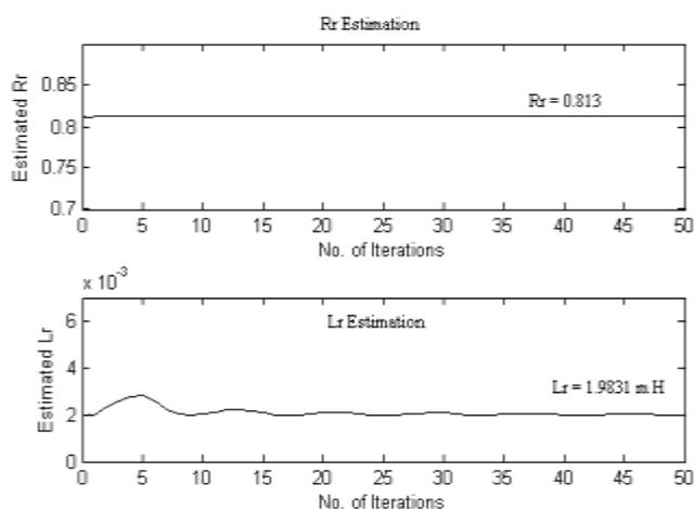
**Fig 6 Estimated values of rotor resistance & inductance (Three bar Broken case)**
