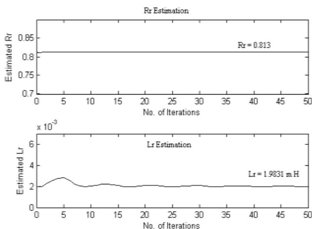
**Fig 5 Estimated values of rotor resistance & inductance (One bar Broken case)**
