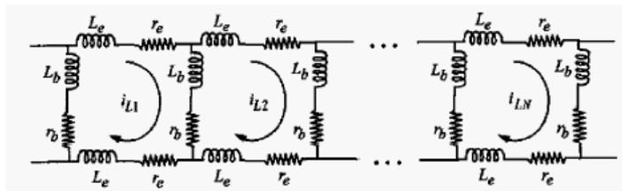
Fig.3 Developed Squirrel Cage Rotor Model
