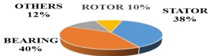
Fig. 2 Classification of faults
