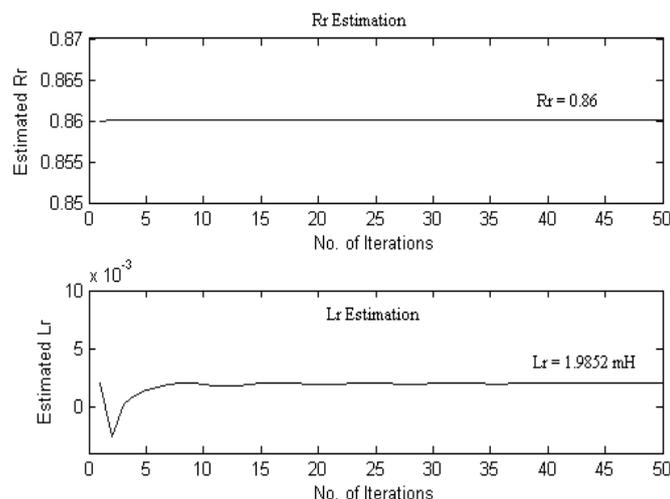
**Fig 7 Estimated values of rotor resistance & inductance (Five bar Broken case)**
