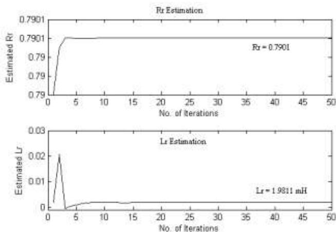
**Fig 4 Estimated values of rotor resistance & inductance (Healthy case)**
