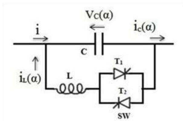
Fig. 1.1: Basic Thyristor Controlled Series Capacitor
