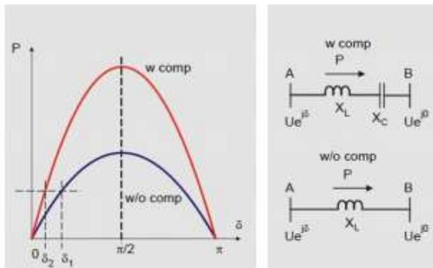
Fig:1.3 Line with Rated Voltage Amplitude in Both Ends
