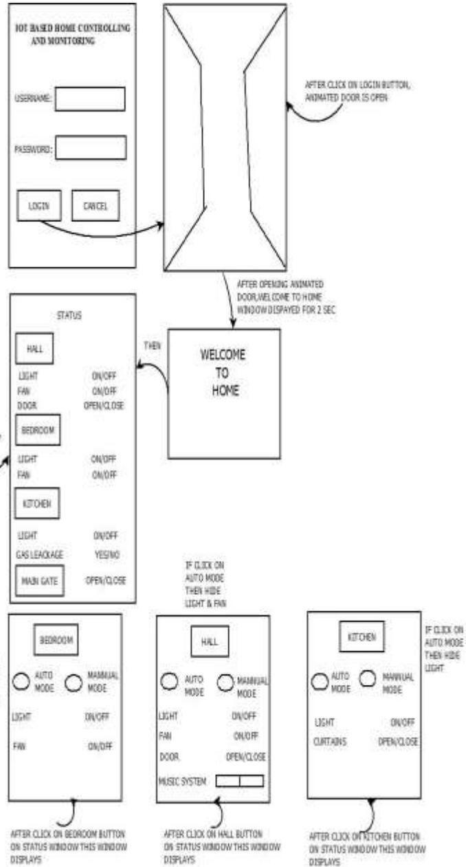
Figure 3: Detailed Block Diagram 2-Home Automation using IOT
