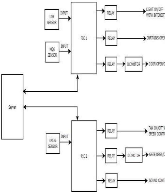
Figure 2: Detailed Block Diagram 2-IOT connected to external sensors & Devices
