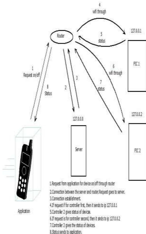
Figure 4: How communication between various devices taking place
