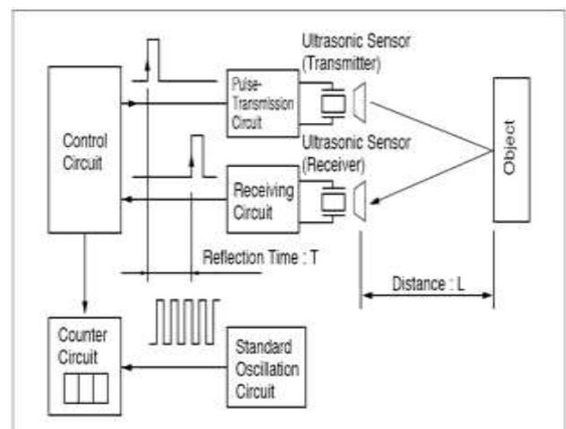
Fig.6. Sensor Detecting the Obstacle
