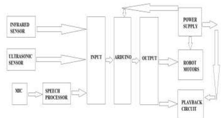
Fig.1. Block diagram of the speech recognition and obstacle detector
