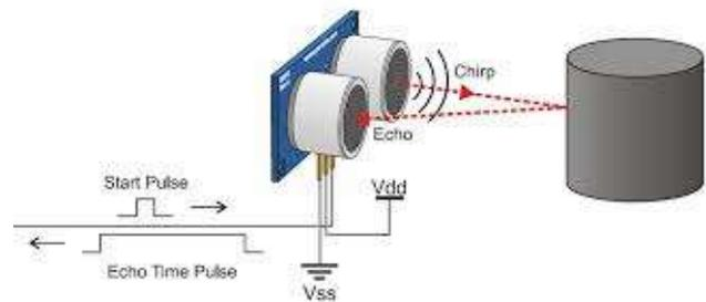
Fig.5. Ultrasonic Sensor operation
