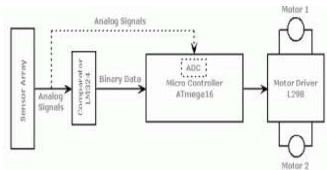
Fig.7. Interfacing the IR sensor to drive the Motors
