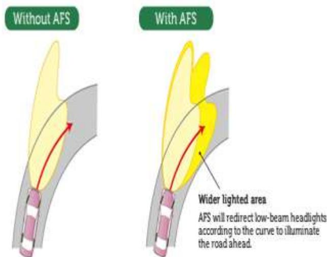
Figure 3.1 Vehicle with adaptive headlight and without advanced headlight
