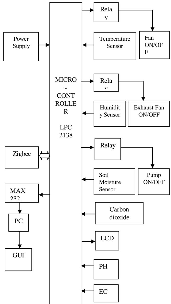
Fig 2. Block diagram of polyhouse automation
