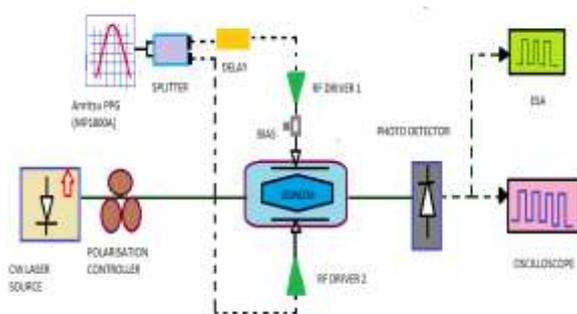
Figure .1. Setup of the reconfigurable UWB pulse generation using DDMZM.
