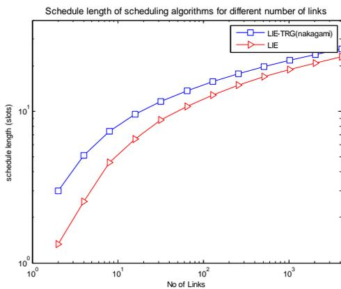
Fig 5.1: Schedule length of scheduling algorithm for different number of links.
