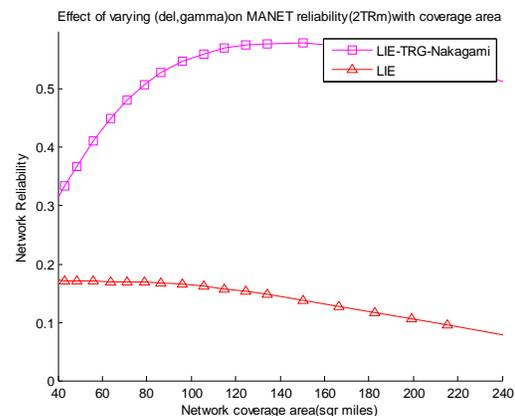
Fig 5.3: Effect of varying (Del, gamma) on MANET reliability (2TRm) with coverage area.
