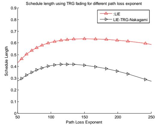
Fig 5.2: Schedule length using TRG-fading for different path loss exponents on network coverage area.
