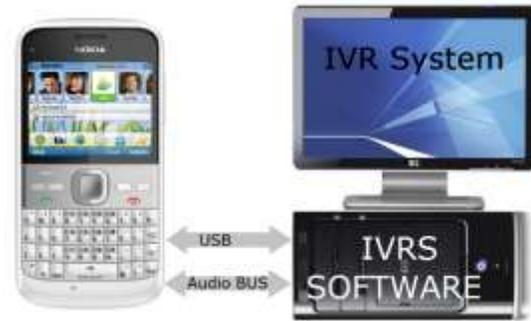
Figure 6: Proposed IVRS Software Architecture
