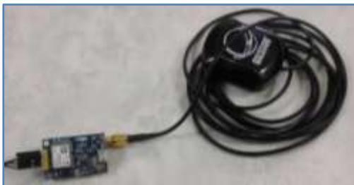
**Fig. 3.Arduino GPS Shield**
