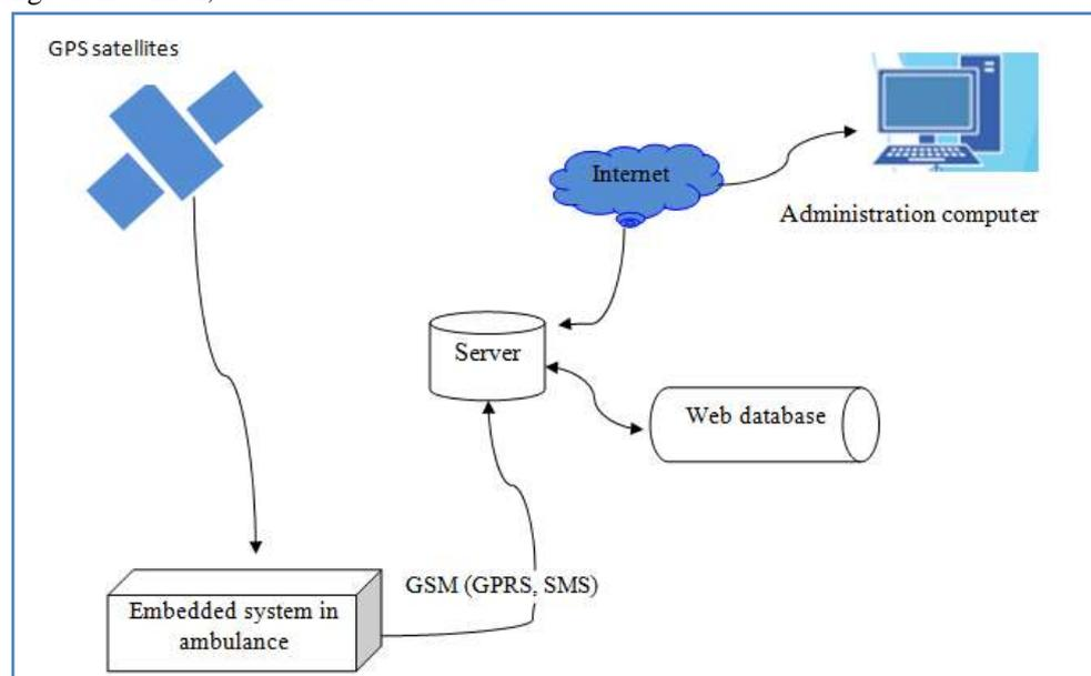
Fig. 1. System design architecture.
