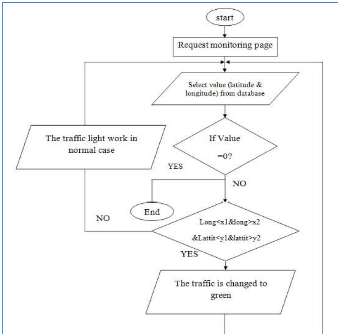
Fig.6 Flowchart of the traffic light control algorithm.
