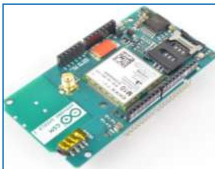
**Fig. 4.Arduino GSM Shield.**
