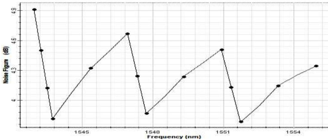
Figure3(b):Upstream noise figure curve
