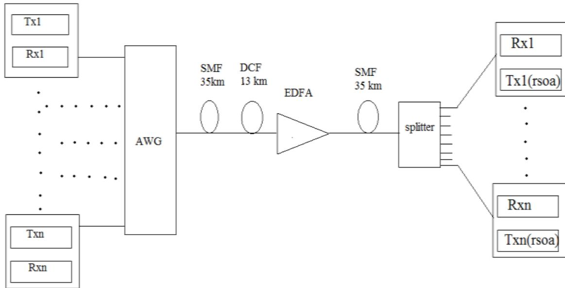
Figure 1: RSOA based WDM PON Architecture
