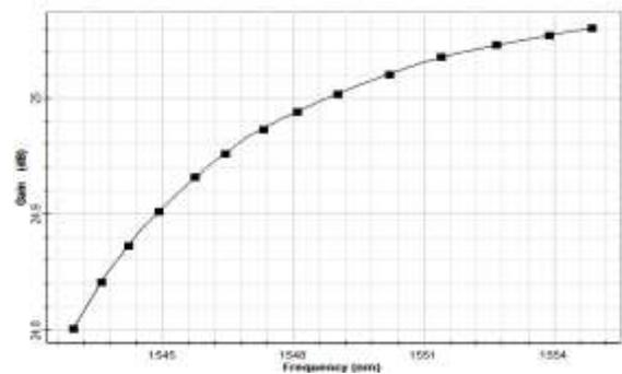
Figure 2(b): Upstream gain curve
