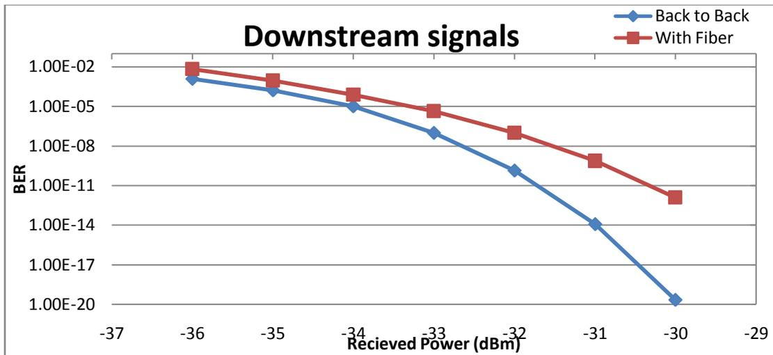
Figure 4(a): BER versus received Power curve for downstream transmission
