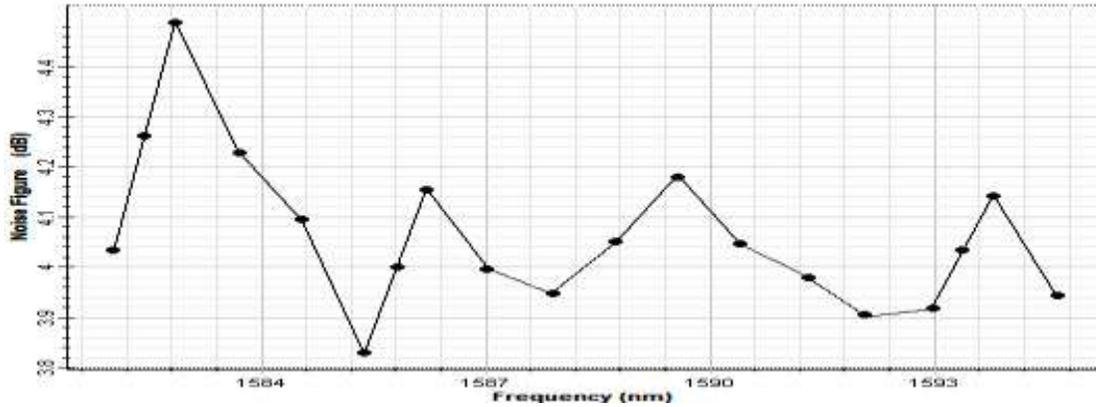
Figure 3(a):Downstream noise figure curve
