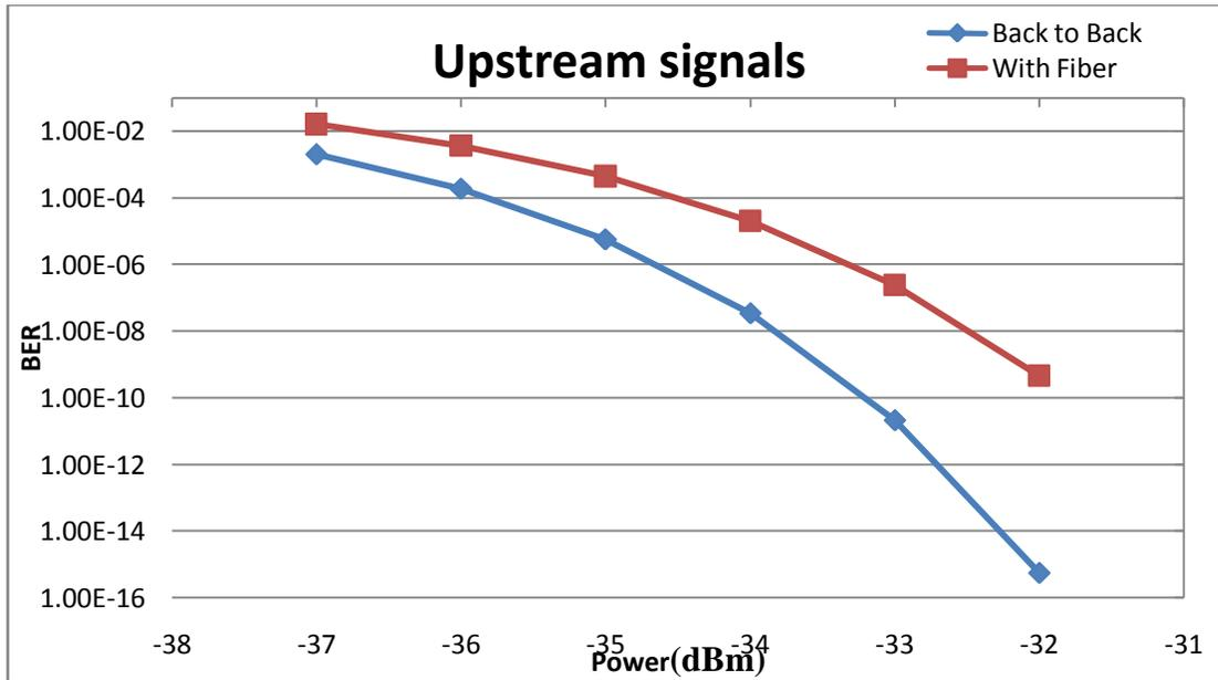
Figure 4(b): BER versus received Power curve for upstream transmission
