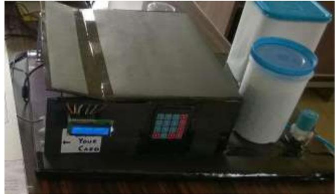
Fig 4: Automated ration distribution System
