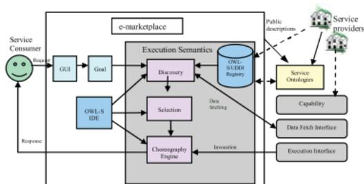
Fig 3. System architecture
