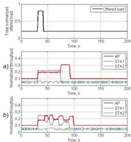
Fig. 1. Normalized total throughput of the wireless network that contains 2 stations and works using a) DCF or b) EDCA access scheme
