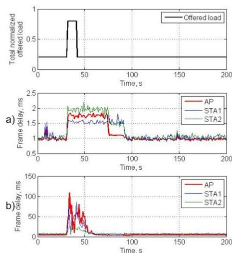
Fig. 2. Mean frame delay respectively for a) DCF and b) EDCA access scheme
