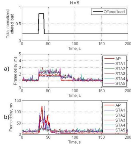
Fig. 6. Mean frame delay for a network of 5 stations in case of using a) DCF and b) EDCA access scheme
