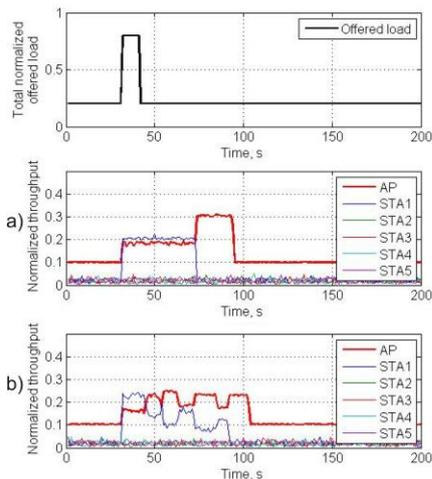
Fig. 4. Normalized total throughput of the wireless network that contains 5 stations and works using a) DCF or b) EDCA access scheme
