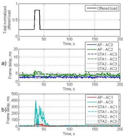
Fig. 3. Mean frame delay for a) high priority and b) low priority frames
