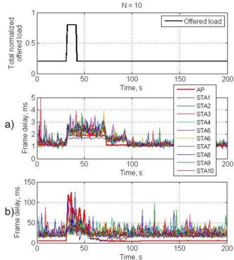
Fig. 7. Mean frame delay for a network of 10 stations in case of using a) DCF and b) EDCA access scheme
