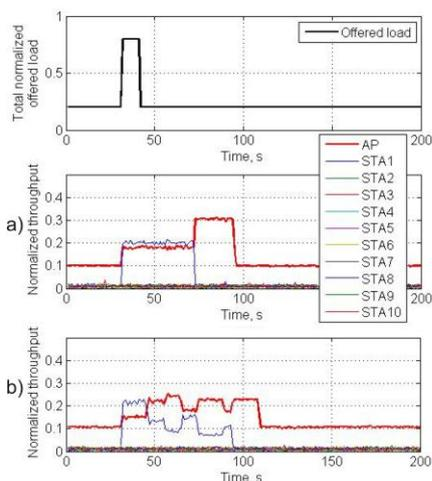
Fig. 5. Normalized total throughput of the wireless network that contains 10 stations and works using a) DCF or b) EDCA access scheme
