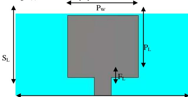
Fig.1 (b).Top View of the proposed antenna
