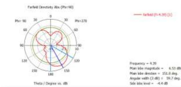
Fig.7.HPBW plot of the proposed antenna
