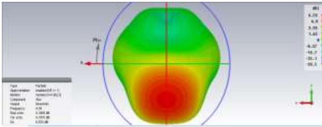
Fig.4.3D plot of directivity for the proposed antenna
