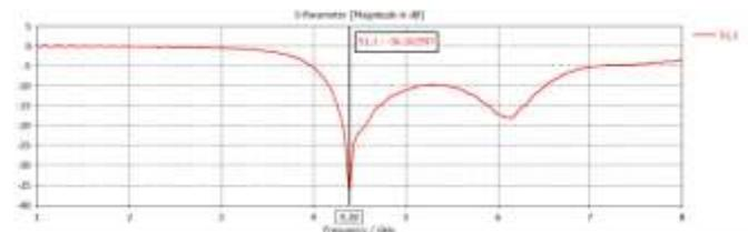
Fig.2.Return Loss plot of the proposed antenna
