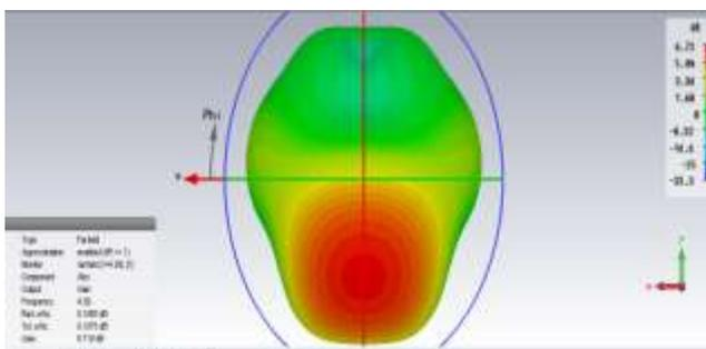
Fig.5.3D plot of gain for the proposed antenna
