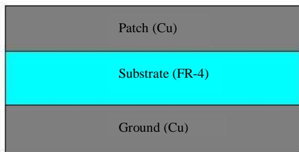
Fig.1 (a).Side view of the proposed antenna
